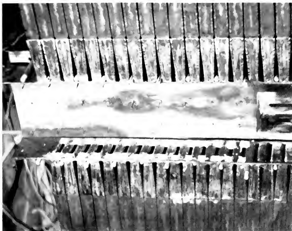
Figure 9 - Close-up of Modified Lower Injection Orifices.
